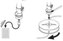
· Screw the trimmer head onto the shaft.
